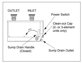
Figure 6. Hydro-Heater Side View
